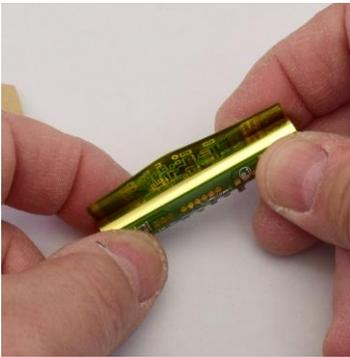
Now wrap the flexible circuit board all the way around the pen tube pressing tightly as you go to ensure that no air is trapped under the sheet.
