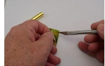
Peel off some of the backing material so you can adhere the sheet to the tube in a straight line.
