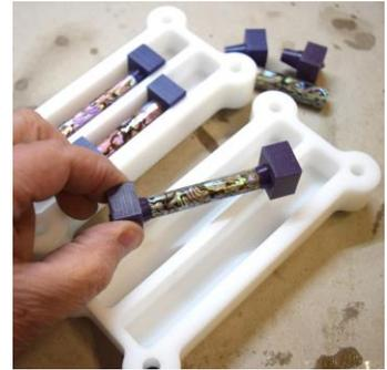
**Step 3** – Firmly press your pen tubes with the silicone plugs in each end into the mold chamber. Make sure it is firmly seated in the bottom of the mold.
