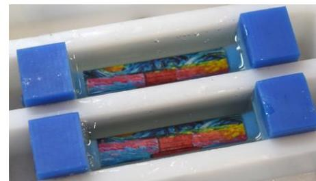
**Step 7 – Demolding:** Once the resin is dry, carefully pull the silicone plugs apart from the pen tube and then simply pull the casted piece out from the mold.
