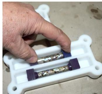
**Step 4** – Mix your resin according to the manufacturer's instructions. Three (3) ounces of resin was thoroughly mixed and then carefully poured into the mold filling each chamber. Take care not to overfill the chambers.
