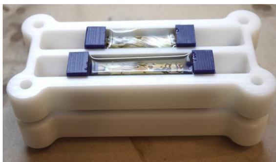
**Step 6** – Here are the two DogBone molds filled with resin. **Please Note:** only 1.5 ounces were used to fill all four chambers and you can see the remaining resin in the cup. In fact, enough resin was leftover to pour two more Sierra Grip pen tubes that have pictures wrapped around the pen tubes.
