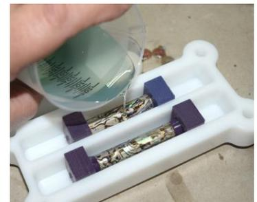
**Step 5** – If any air bubbles appear, tease them to the surface. Also, if using a pressure pot and more than one mold, stack them and place into pressure pot. Polyester resin was used for this example so a pressure pot was not needed.
