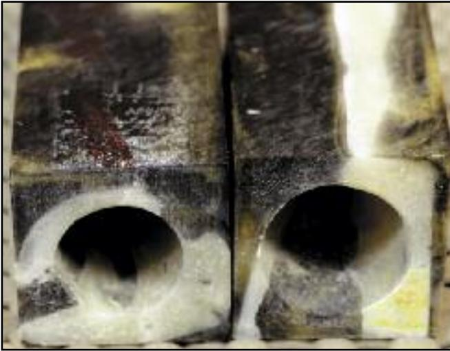
**Step 7.** This is a comparison of the entry hole on the left and the exit hole on the right. See how clean both holes are by using a combination of the appropriate speed; a sharp, lubricated drill bit; and a constant feed rate while relieving the debris consistently.
