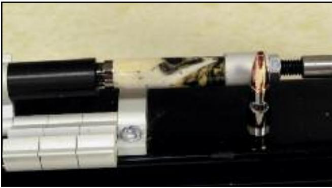
**Step 25.** Unscrew the nib section, leaving behind the nib coupler. Carefully move it to the pen press and press it into the barrel. Press the finial end into the other end of the barrel to complete the lower barrel assembly. Once you screw the nib section back on and screw it into the cap section, it should line up. Your Alligator Jaw Bone Pen is finished—now that did not take a bite out of you, did it?
