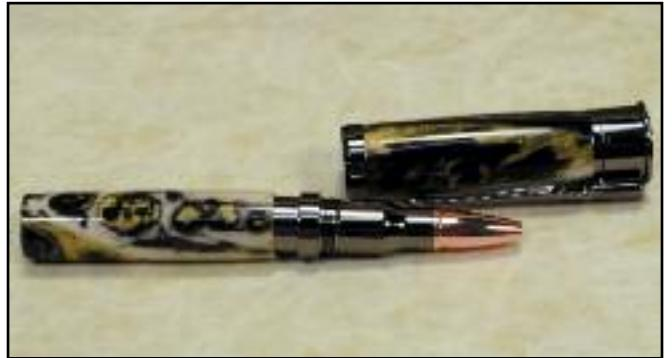
**Step 23.** Screw the rollerball nib section into the nib coupler and loosely push it into the lower barrel.
