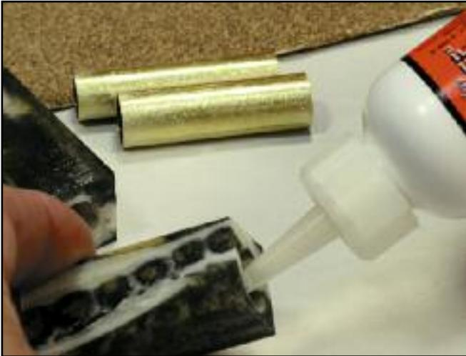
**Step 8.** Place a light coating of thin cyanoacrylate glue (CA or superglue) into both pen blanks to soak into the jaw bone for additional strength. Use medium CA and glue in the pen tubes that were roughed up in Step 4. You can use 5-minute epoxy here as well—it just takes longer to dry.
