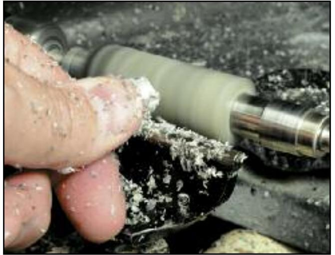
**Step 10.** These blanks do not require carbide-tipped tools, so start with a roughing gouge taking LIGHT CUTS and reduce the blank down close to the bushings. (My definition of light will be different than yours, but please take very light cuts.)
