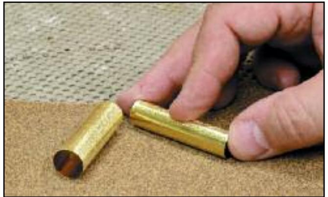
**Step 4.** Rough-up the pen tubes so that the glue will have a good bonding surface with the tube and the inside of the alligator pen blank.
