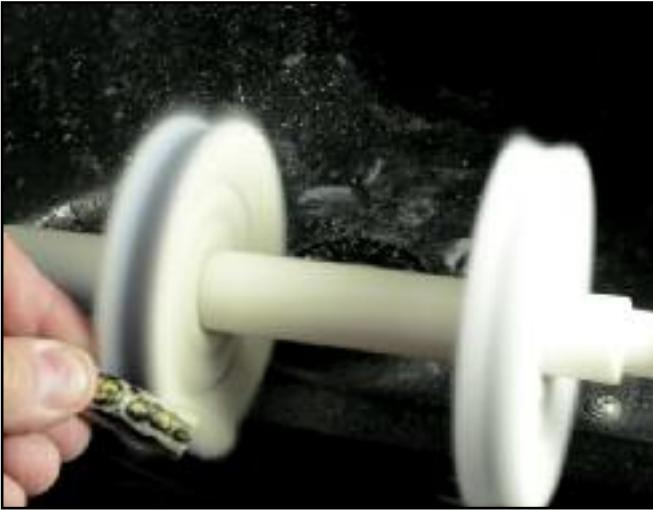
**Step 19.** Buff the blank using the acrylic pen buffing system with the special blue rouge designed specifically for acrylics. Repeat the process for the other half of the alligator blank.
