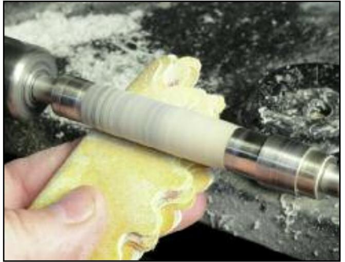
**Step 16.** Put the blank back onto the mandrel and sand it with abrasive paper, starting at 180 or 220 grit because you already had it fairly smooth with the skew. Sand up to 800 grit.
