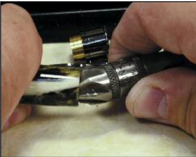
**Step 21.** Use a chamfering tool on the inside of the brass tube to break the sharp edge. This will aid in assembly when the pieces are pressed into the tube and will reduce the number of "cracks" on the ends of the pen.
