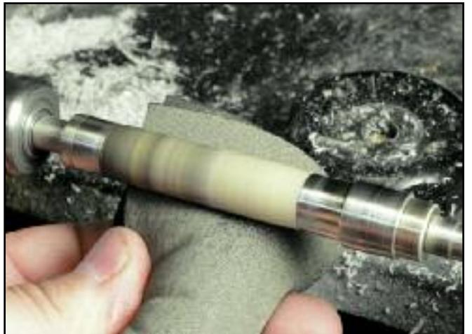
**Step 17.** After the 800 grit, sand with the four Abralon pads to 4,000. The Abralon pads use a different grit system, so the 4,000-grit pad is equal to the 12,000 grit from other manufacturers.
