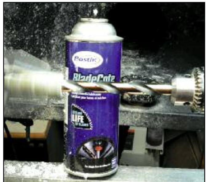
**Step 6.** Drill the blank at around 1000 rpm with a Norseman 9/16" bit for the upper tube and a Norseman 12.5mm bit for the lower tube. *Hint:* I only use a drill chuck to drill all my pen blanks and spray the drill bits with Bostik BladeCote before drilling. The BladeCote reduces friction and keeps the drill bit sharper longer!
