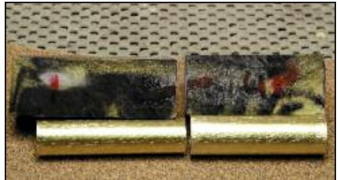
**Step 5.** Make sure that you mark the blank by putting an orientation line on the blank so that you know which half of the blank is the upper and which one is the lower. Doing so will ensure that the tooth holes line up.
