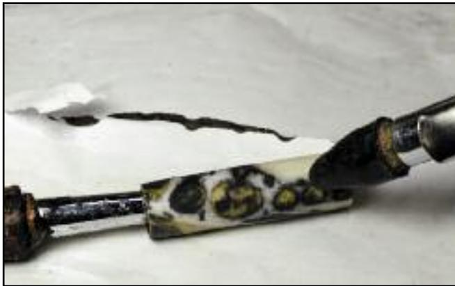
**Step 14.** Use compressed air to blow out any debris that might remain after taking a final pass with the skew.
