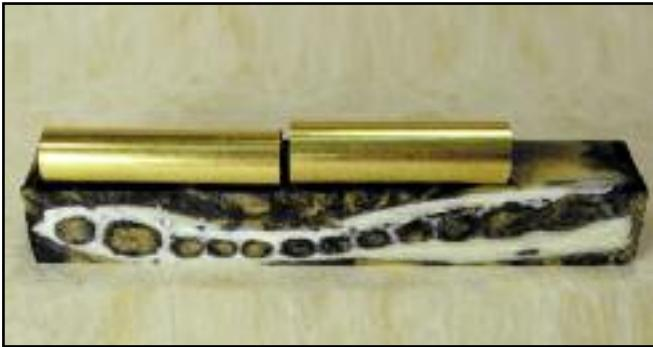
**Step 2.** Lay the pen tubes on the pen blank and align the tubes so that you get the most tooth holes showing within the pen blank.
