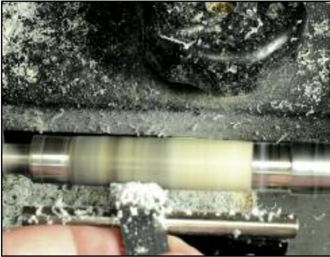
**Step 13.** Use a skew to reduce the blank down to the bushings, and then use the skew as a scraper for a final pass.
