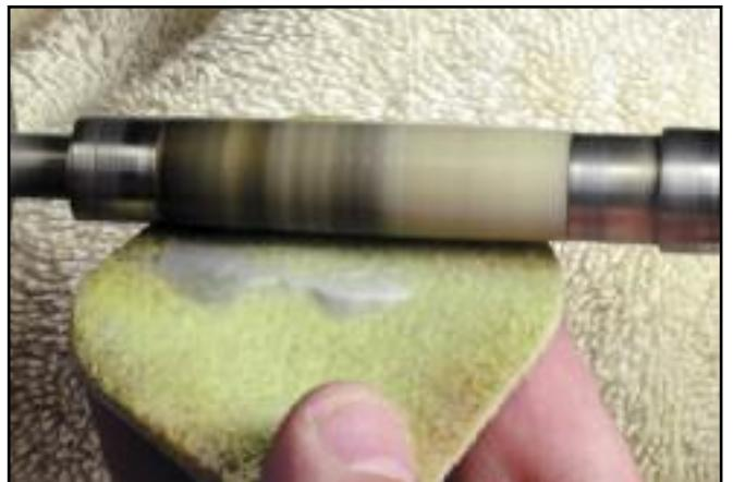
**Step 18.** Wet-sand the blank using the acrylic finishing pads.
