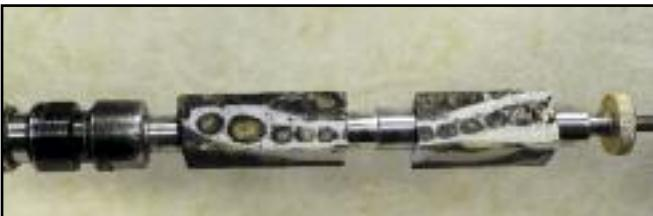
**Step 9.** Place the pen tubes onto the mandrel with the appropriate bushings. *Note:* Make sure that you have the blank lined up so that the teeth are showing in the proper direction! Both blanks have been placed on the mandrel just for visual purposes—I only turn one blank at a time!
