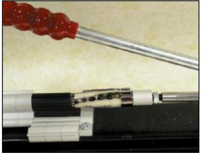
**Step 22.** Start with the upper barrel of the pen, and press the clip and then the centerband into the upper blank.
