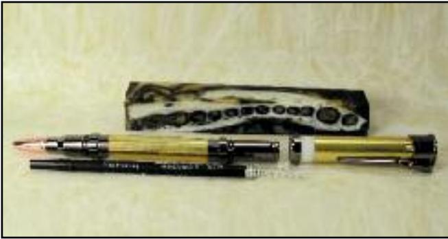
**Step 1.** Remove the pen parts from the plastic bag and line them up according to the manufacturer's instructions. For this project, I am using an Over/Under shotgun rollerball pen kit with the Black Lava Swirl Alligator Jaw Bone Pen Blank.
