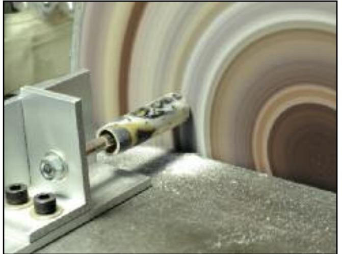
**Step 11.** Once the blank is reduced close to the bushing diameter, square the ends of the blank. I do not use a barrel trimmer for this purpose—I use a squaring jig. I always reduce the blank almost flush to the bushings before squaring the ends—by doing it this way, only a small amount of material is removed, rather than trying to surface a large square piece.
