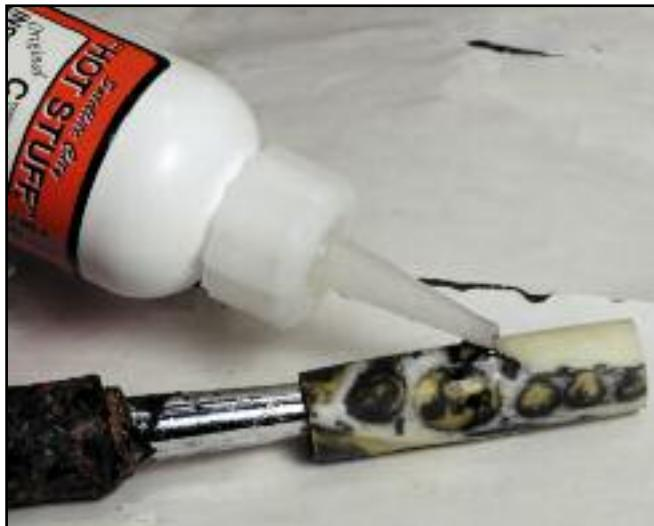
**Step 15.** Drip thin CA over the entire blank to fill in any small hairline openings that the jaw bone may have (this is natural because it is a biological product). The CA will also give additional strength to the piece.
